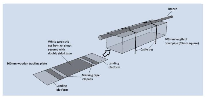
Figure 4. Footprint tunnel design showing the arrangement of card and ink pads on the wooden tracking plate, which is inserted into the shorter tunnel made of square downpipe.
